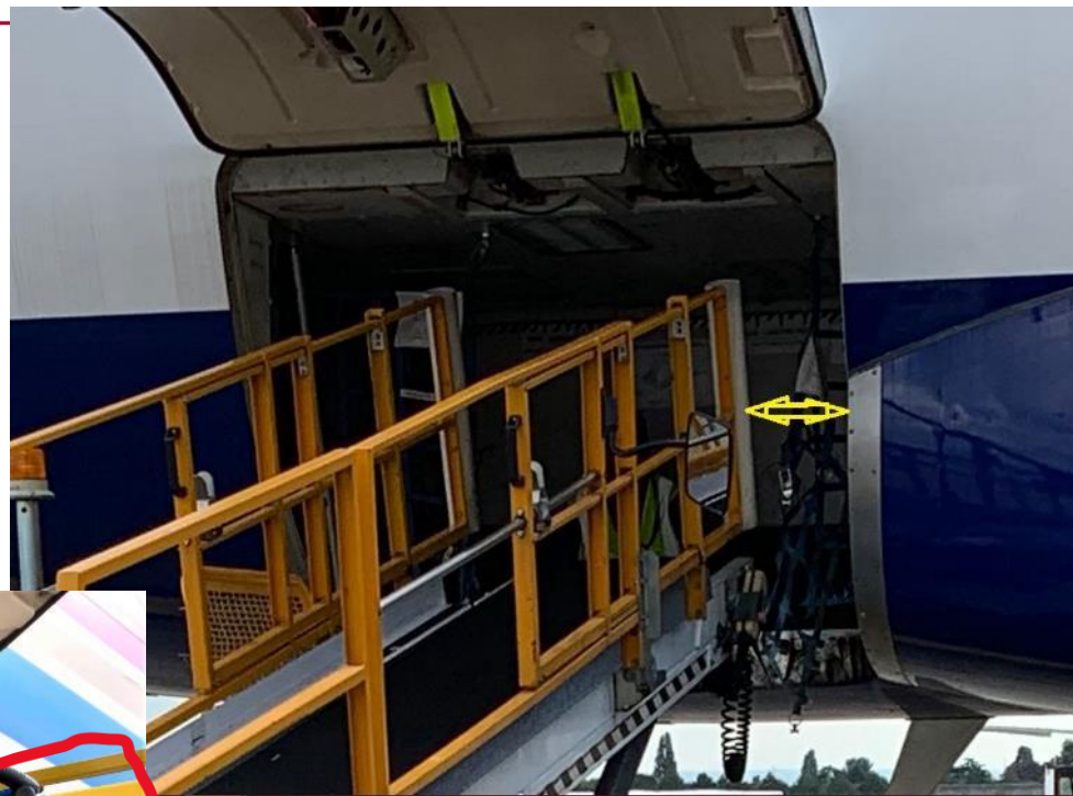
Gap between loader and cargo doors
