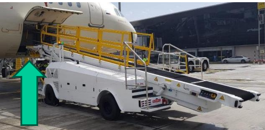
Large gap between handrail and loader
