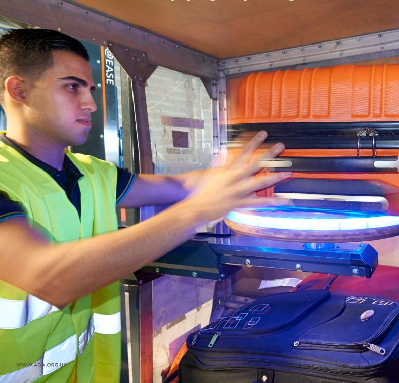
ollowing testing at Terminal 3 and Terminal 5, Vanderlande has supplied and installed 72 STACK@EASE units as part of the terminal's integrated baggage system. The new facility is the most advanced baggage system in Europe with a baggage handling capacity of up to 7,200 bags per hour. The system is designed to cut the time it takes to get bags ready for a flight to 90 minutes or less. Heathrow handles over 185,000 bags a day through a system comprising 30 miles of conveyors.
