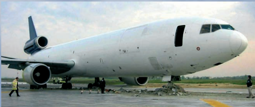
MD-11 EMAS arrestment with minimal injuries or damage to aircraft. Photo courtesy of the Port Authority of NY & NJ
