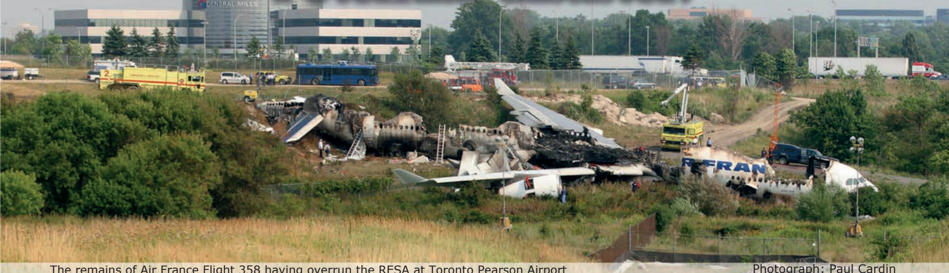
The remains of Air France Flight 358 having overrun the RESA at Toronto Pearson Airport
