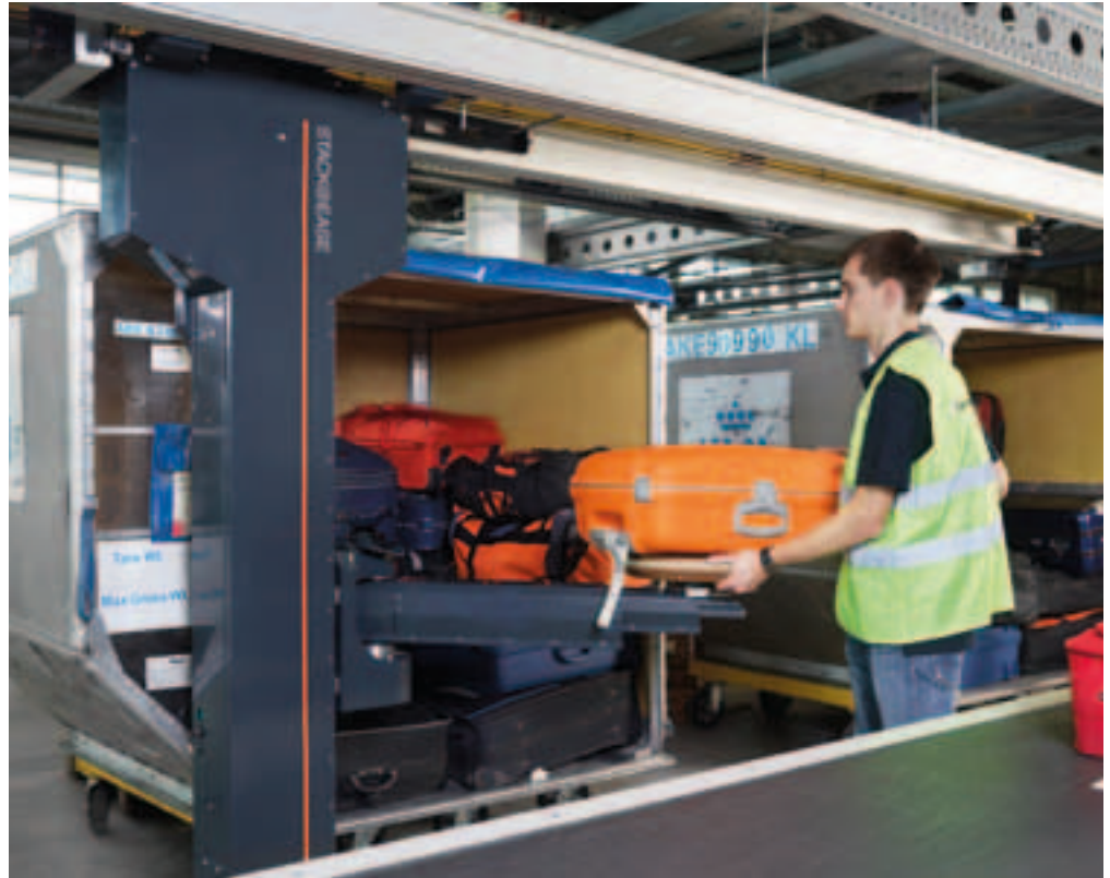
In addition to significantly improving working conditions for baggage handlers, one of the main benefits of Vanderlande's STACK@EASE compact manual handling aid is increased productivity for airports of all sizes. Its use is not limited to large airports, but is an effective option for smaller airports too, for application where and when it is needed.
