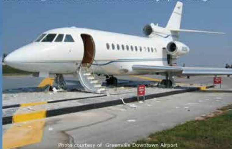
EMASMAX ® arrest of Falcon 900 without injury or damage.
